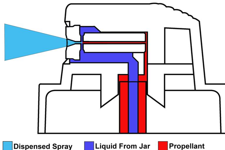
Preval has a proprietary technology that makes a highly controlled atomized spray from any liquid. When the button is pressed, propellant and liquid are mixed and dispensed as a spray at the nozzle by action of the venturi effect. Liquid from the jar is pulled up the tube as propellant travels across the holes in the red insert (inside the button). The propellant and liquid do not mix prior to being dispensed out of the nozzle.
