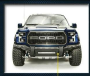
MADE FROM 11-GAUGE U.S. STEEL WITH 1.75X.120-INCH WALL TUBING
